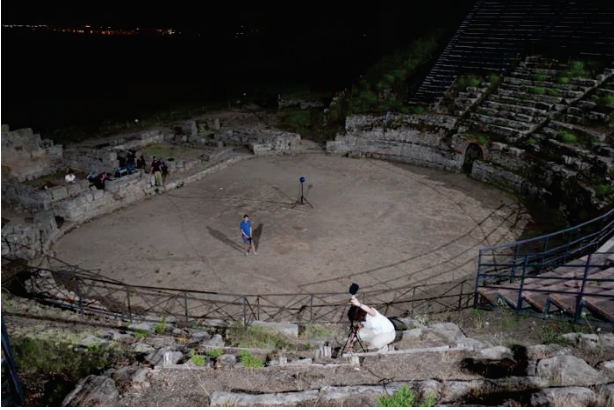
Figure 7. Example of measurement: sound source in position S1 and receiver in position R3.
